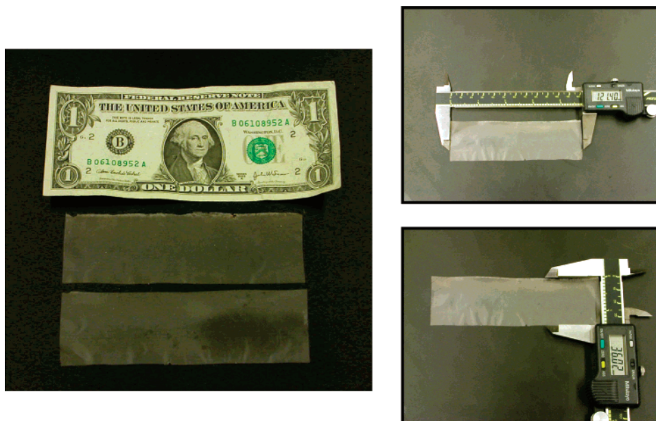
Figure 8. Large-area free-standing LbL-assembled (HM-PEO35K/PAA) 60 multilayer film.
